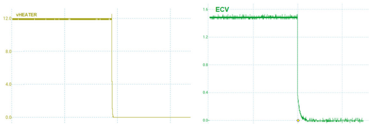
Figure 17. Heater and ECV outputs switch-off curves
