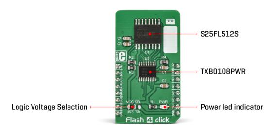
The advanced MirrorBit® technology allows storing of two data bits in each memory array transistor (memory cell), effectively doubling the capacity of a single storage cell this way. The Eclipse™ architecture is responsible for the greatly improved erase and programming performance, compared to other Flash modules of the previous generation. Due to a higher speed, an execute-in-place (XIP), as well as the data shadowing is possible with the Flash 4 click.
