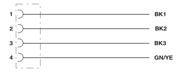
Contact assignment of the M12 socket
