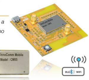
CM05, BLE WiFi Combo module, is comprised of BLE and WiFi technologies with an ARM® Cortex-M4 MCU to run customer's IoT applications.
