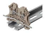
With the LS 2.8 WDU2.5-10, many feed-through modular terminal blocks from the W series can be converted very easily. Inserting the LS 2.8 WDU2.5-10 allows the cable shielding braid to be looped through directly at the terminal block by soldering or using a suitable flat cable lug.
