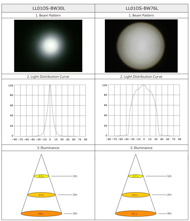
Notes: The Flux of Osram W5AM LED is 80 lm
