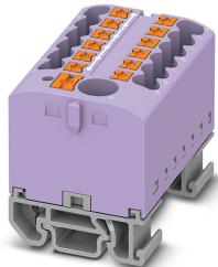
Distribution block, Block with horizontal alignment and integrated supply, the blocks can be bridged with one another via the conductor shaft, for corresponding plug-in bridges, see accessories, nom. voltage: 690 V, nominal current: 24 A, connection method: Push-in connection, Push-in connection, number of connections: 13, cross section: 0.14 mm<sup>2</sup> - 4 mm<sup>2</sup>, AWG: 26 - 12, width: 41 mm, color: violet, mounting type: NS 15
