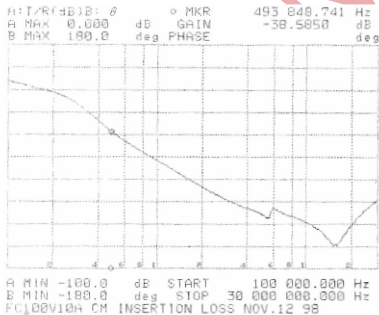
Figure 9 - Common Mode Attenuation Plot
