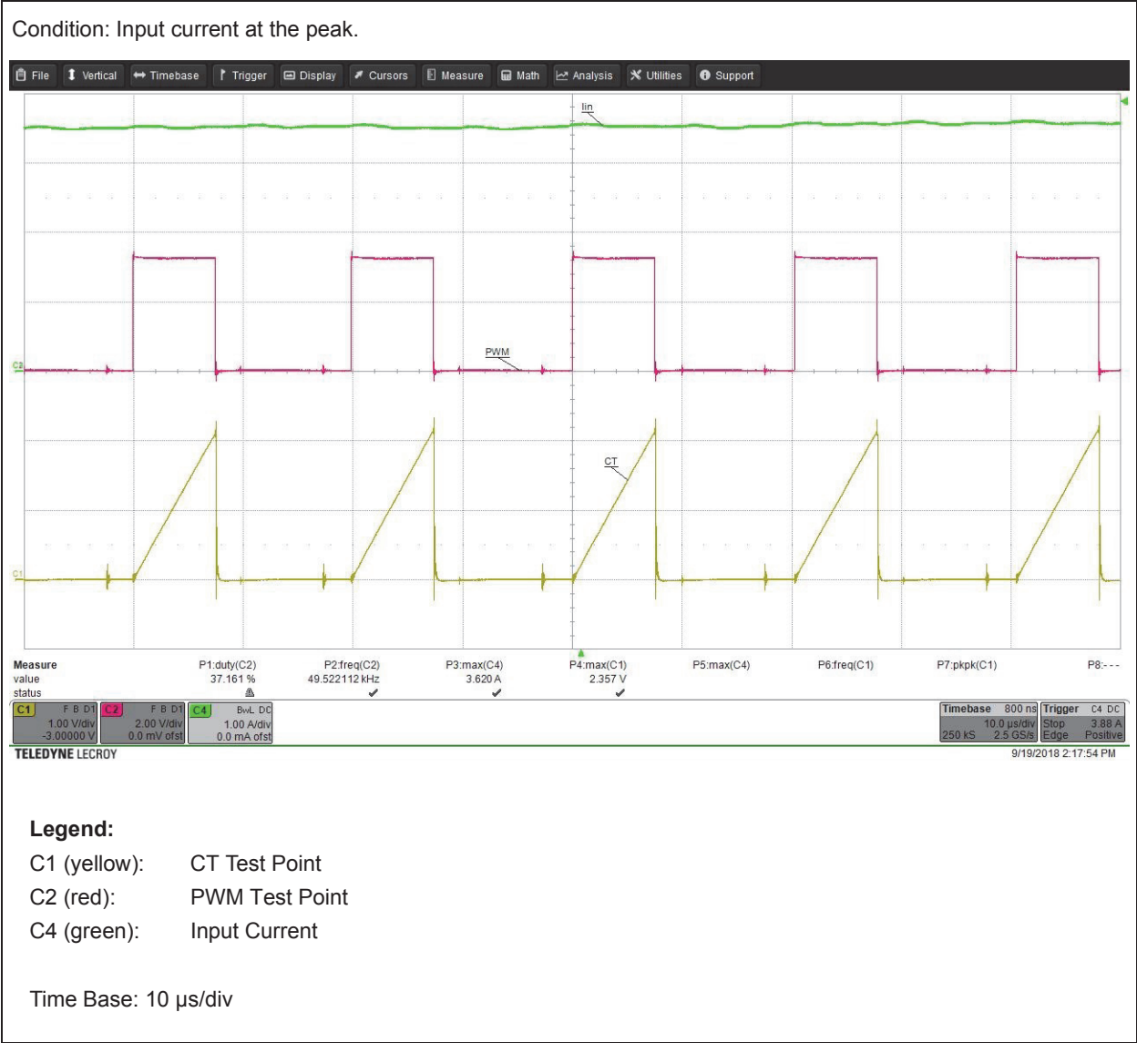
FIGURE 1-12: CURRENT TRANSFORMER (CT), PWM TEST POINTS
