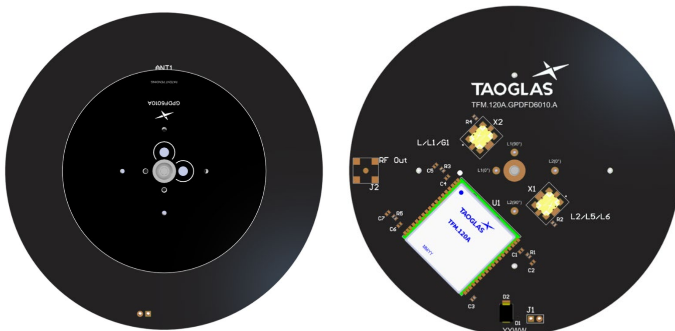
Top and bottom view of PCB.
