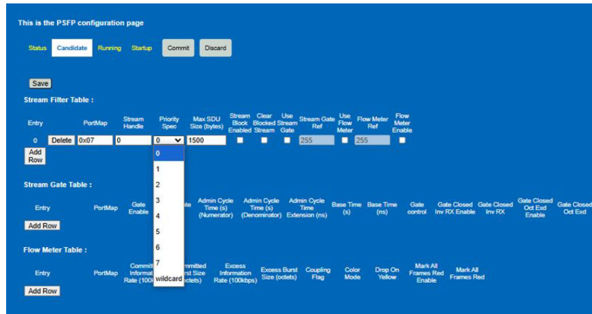
Figure 151. Stream Filter Configuration
