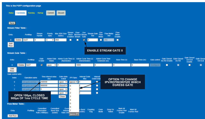
Figure 153. Stream Filter and Stream Gate
