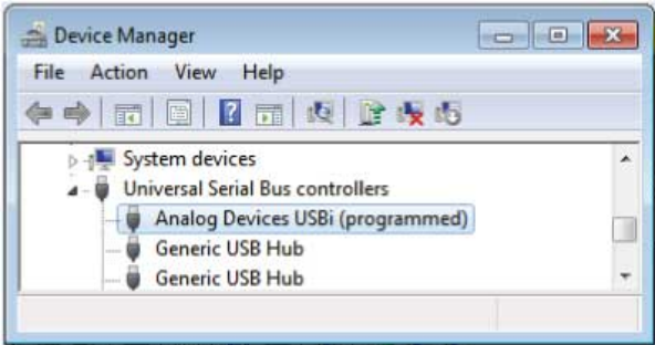
Figure 9. Confirming Driver Installation Using the Device Manager
