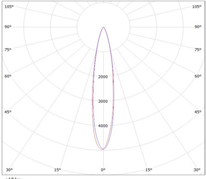
cd/klm \_\_\_\_\_\_ C0 - C180 \_\_\_\_\_ C90 - C270 Luminaire: Ledil Oy CA11355\_LAURA-M\_(3535\_Ceramic\_gen2) Efficiency=82% Lamps: 1 x LG 3535 Ceramic gen2 (PKG5700K) 116Im @ 250mA CCT=6200K P=0.7W I=250mA
