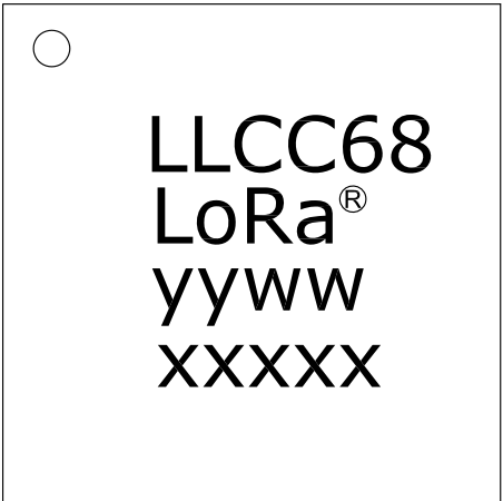
Marking for the 4 x 4 mm MLPQ 24 Package nnnnnn = Part Number yyww = Date Code xxxxx = Semtech Lot No.
