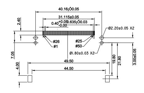
General Tolerance +/-0.05mm **Recommended PCB Pattern**
