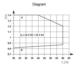
Curve A Maximum permissible continuous voltage  $U_{\text{max}}$  with limiting continuous current on the contact side (see relevant technical data)
