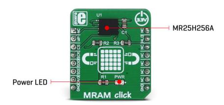
The #HOLD pin of the MR25H256 IC is routed to the INT pin of the mikroBUS™ and it is used to hold the data transfer. When this pin is pulled to a LOW logic level, all data transfer operations
