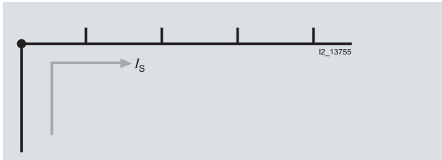
Infeed at the start or end of the busbar
