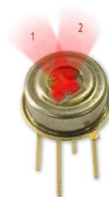
Figure 29 – Typical FOV of MLX90614xBA, Zone 1 & 2 identification relative to the alignment tab
