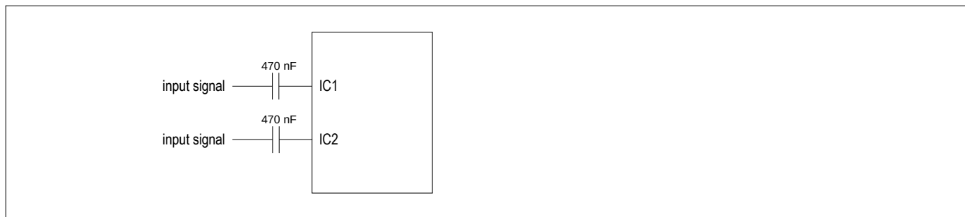
Figure 9-1. Recommended External Components for AMI Composite Clock Pins
