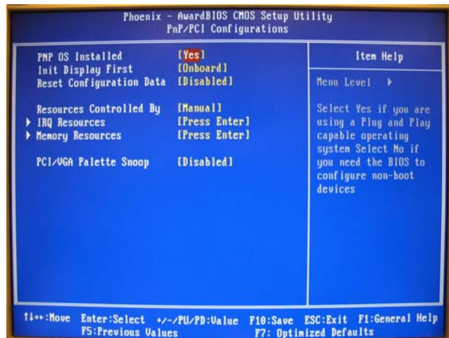
Figure 3.4: PnP/PCI configurations screen
