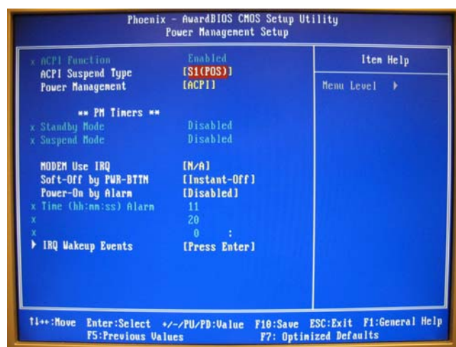
Figure 3.3: Power management setup screen
