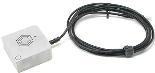
The Touch Probe from Carbide 3D is a small accessory piece for your Shapeoko CNC machine meant to assist in finding the edges, or datums of the part you are milling. This part is an active probe, and when contacted to ground, communicates its position to the Carbide Motion program to help you fabricate easier.
