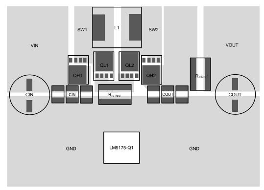
Figure 29. LM5175-Q1 Power Stage Layout
