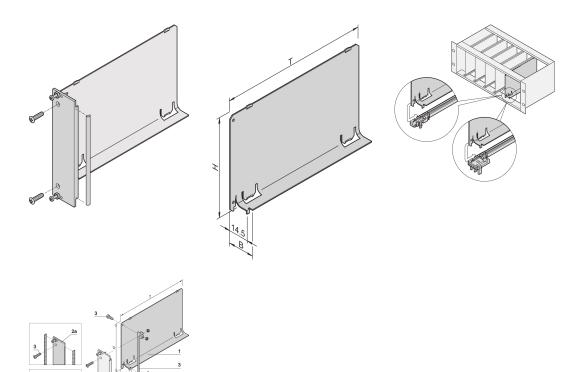
The air baffle with U-shaped front panel covers an empty slot to eliminate an air flow exit. The U-shaped front panel accepts a textile EMC gasket.
