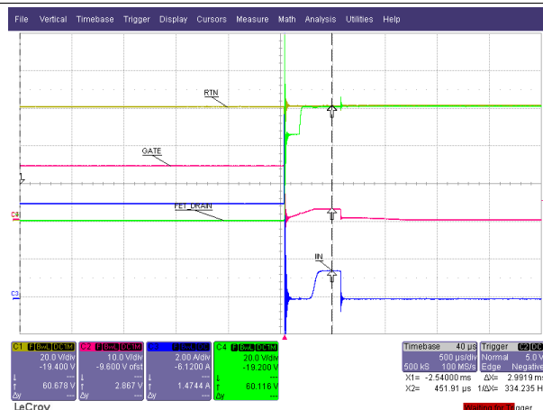
Figure 15. Output Hot Short ( V_{IN}B = 54 \text{ V} )
