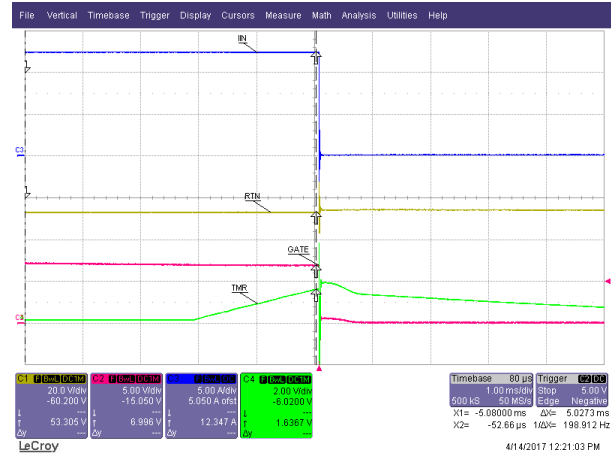
Figure 19. Gradual Over Current ( V_{INA} = 54\text{ V} )
