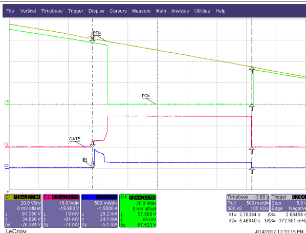
Figure 32. Plug in V_{IN}A Backwards
