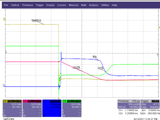
Figure 12. Hot Plug A after B
