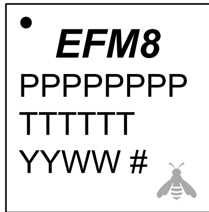
Figure 7.3. QFN28 Package Marking
