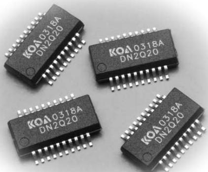
This diode network is designed to provide seventeen channels for active termination of high-speed data signals to eliminate signal undershoot and overshoot. The network has the added benefit of acting to suppress any ESD voltage events by shunting the energy to ground assuring maximum reliability of electronic systems in the field. Trigger levels are defined by the positive and negative bias levels set by the user.
