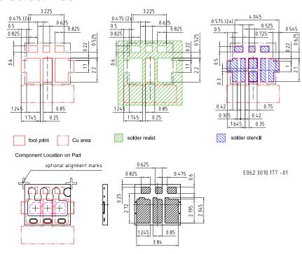
For superior solder joint connectivity results we recommend soldering under standard nitrogen atmosphere. Package not suitable for ultra sonic cleaning. To ensure a high solder joint reliability and to minimize the risk of solder joint cracks, the customer is responsible to evaluate the combination of PCB board and solder paste material for his application.
