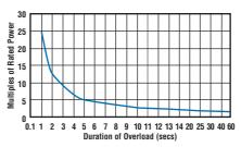
This graph indicates the amount that the rated power (at 20°C) of the standard KHSA Series resistor may be increased for overloads of 100mS to 60S
