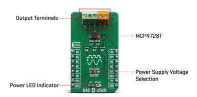
The MCP4728 device has a high precision internal voltage reference (VREF = 2.048V). The internal reference can be selected by user, or external reference may be used (VDD) for each channel individually. This gives the ADC 4 click good flexibility for use in various applications.
