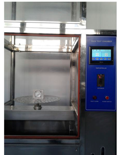
Testing under water jet
