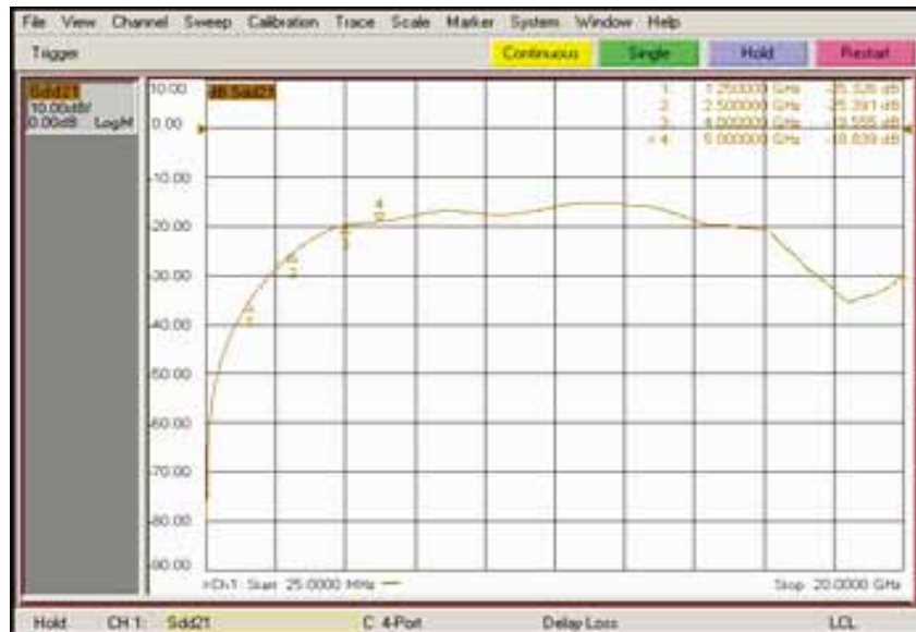
Differential Off Isolation
