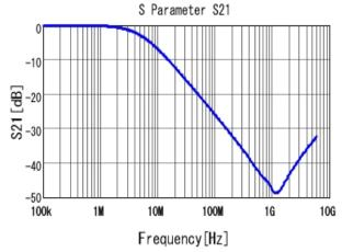
NFM15CC222D1A3 S21 DCOV, 25degC, Feedthrough
