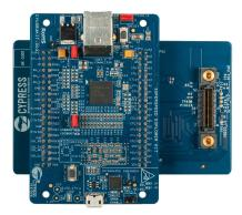
Connect the ON Semiconductor Image Sensor Board (MT9M114\_55CSP\_HB\_DEM03\_REV0) to the CYUSB3ACC-004A Board
