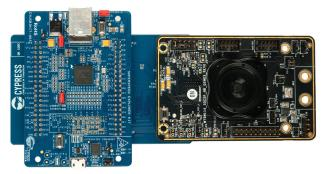
Note : CYUSB3KIT-003 and ON Semiconductor Image Sensor Board (MT9M114\_55CSP\_HB\_DEM03\_REV0) are not part of this kit
