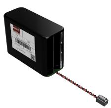
Type DSM Standard Supercapacitor Modules provide a wide range of capacitance values and voltages to enable simple, rapid implementation into any system. Each module features an insulated construction with integrated cell balancing, cable assembly with a Molex Mini-Lock connector, and 85 °C rated supercapacitor cells.
