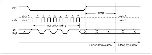
Figure 38a. Release Power-down Instruction (SPI Mode)
