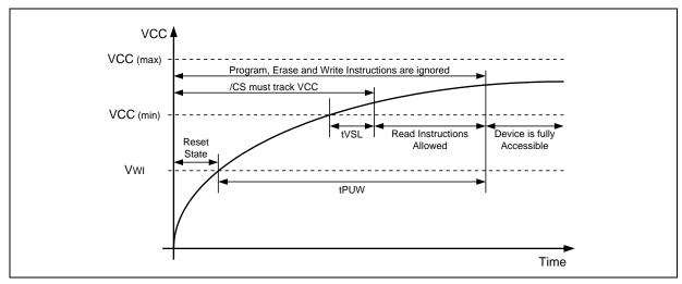
Figure 58a. Power-up Timing and Voltage Levels
