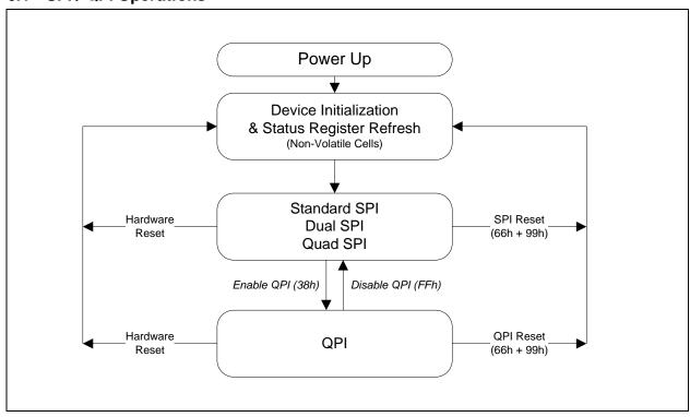
Figure 3. W25Q128JW Serial Flash Memory Operation Diagram
