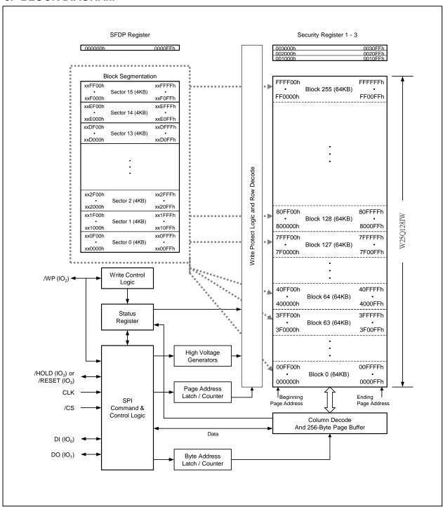
Figure 2. W25Q128JW Serial Flash Memory Block Diagram
