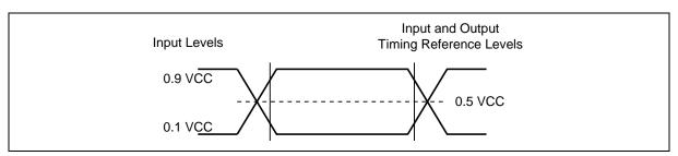
Figure 59. AC Measurement I/O Waveform
