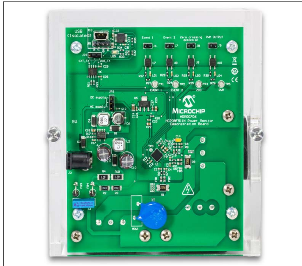
FIGURE 1-1: MCP39F511N Power Monitor Demonstration Board.
