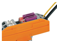
Blown fuse indication via LED
