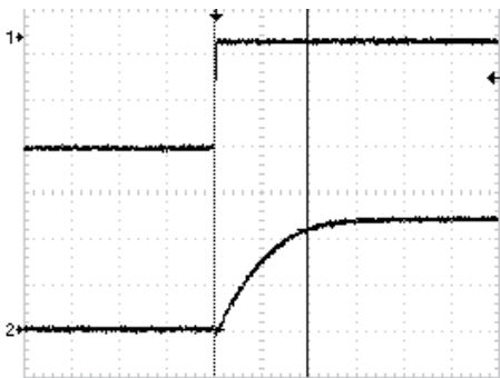
Typical Start-Up Wave Form
