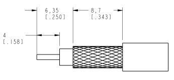
RECOMMEMDED CABLE STRIPPING DIMENSIONS SCALE 3.000
