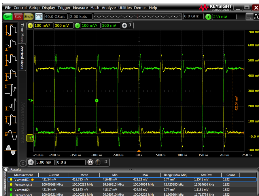
Figure 5-2. HCSL 2.5 V, 100 MHz Clock Measured with DC Coupling, 50-Ω Scope Termination
