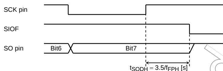
Figure 3.10.27 Transmitted Data Hold Time at End of Transmission
