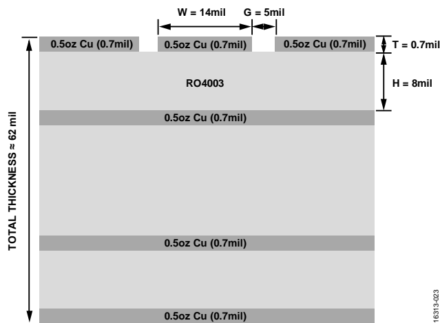
Figure 23. Evaluation Board (Cross Sectional View)
