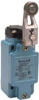
Global Limit Switches Series GLS: Side Rotary With Roller - Adjustable, 1NC 1NO SPDT Snap Action, 0.5 in - 14NPT conduit
