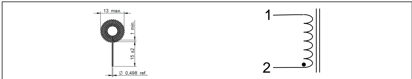
Figure 13 DM choke (side view) and electrical diagram
