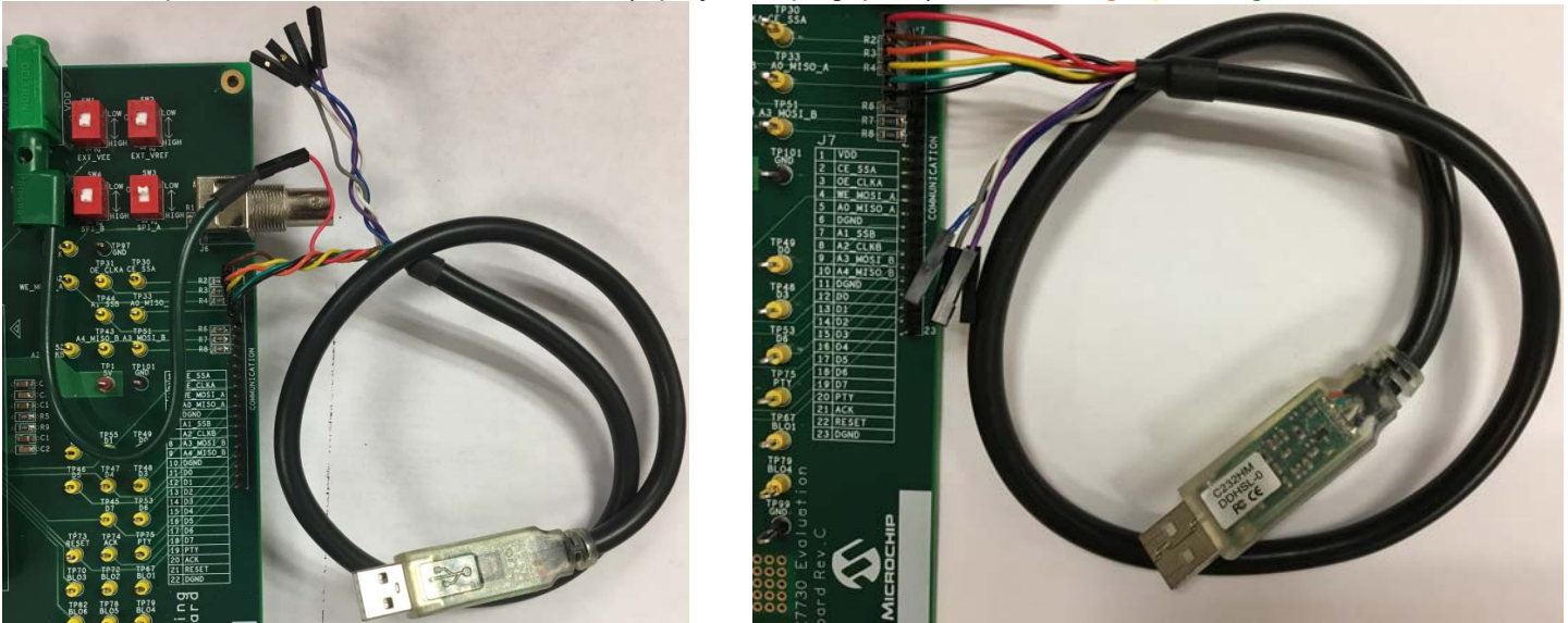
Figure 3. FTDI Dongle's Connections to LX7730-EVB Rev. B board (left), LX7730-EVB Rev. C board (right)
