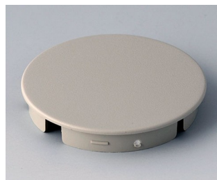
A4140007 Cover 40, without line ABS (UL 94 HB) pebble gray RAL 7032
