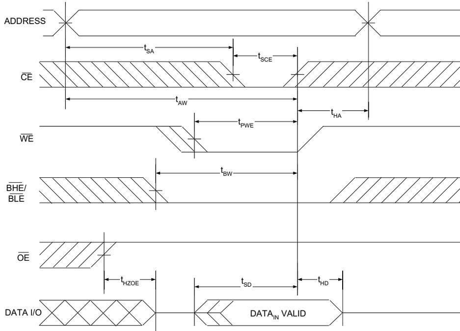
Figure 8. Write Cycle No. 2 ( $\overline{\text{WE}}$  Controlled,  $\overline{\text{OE}}$  LOW) [17, 18, 19, 20]
