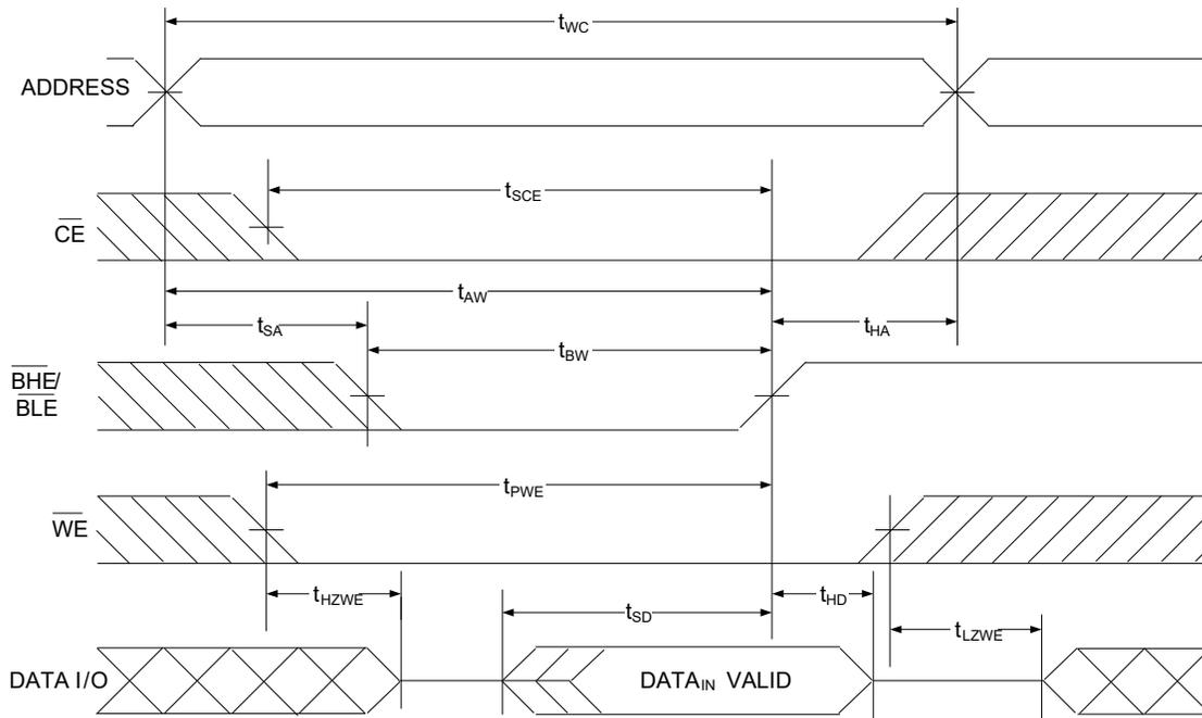
**Figure 10. Write Cycle No. 4 ( $\overline{\text{WE}}$  Controlled) [21, 22, 23]**
