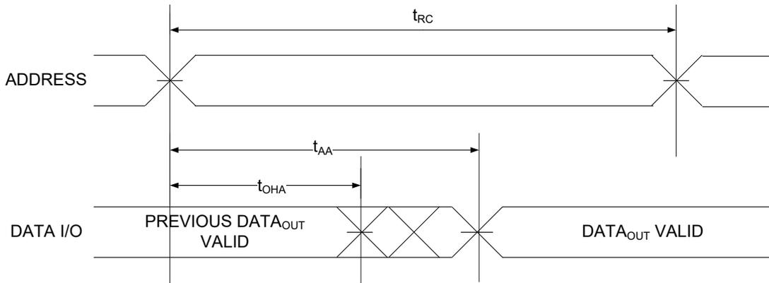
Figure 6. Read Cycle No. 2 ( $\overline{OE}$  Controlled) [16]
