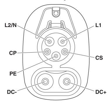
Pin assignment of vehicle charging inlets
