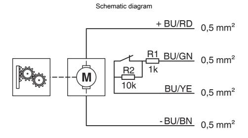
Block diagram of the locking actuator
