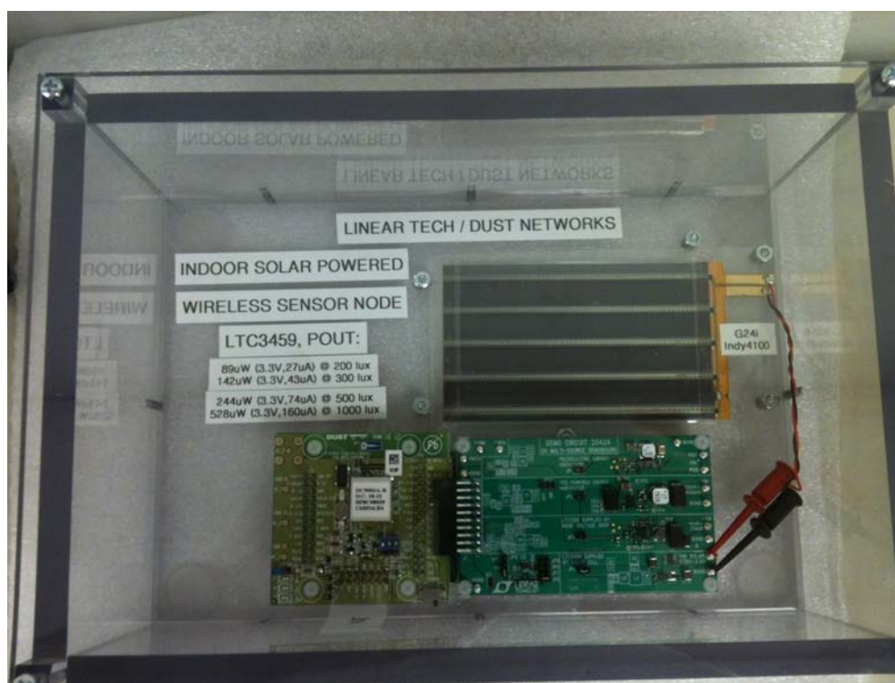
Figure 13. Solar Powered DC2042A in a MESH Wireless Sensor Network
